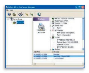
Clicking the "Status" icon on the tool bar will show the status of the currently selected Print Server on the right side of the window. The Print-Server information displayed includes the MAC ID, model type, firmware version, port status, IP address, subnet mask, default gateway, and supported printing protocols.
